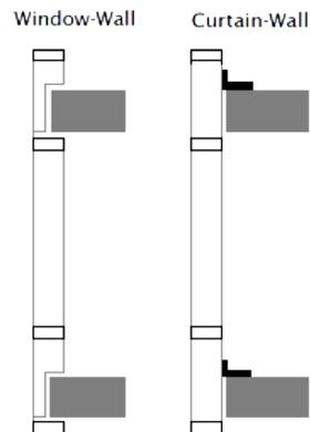
Figure 2: Simplified Window Wall and Curtain Wall
